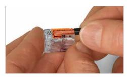
Strip conductor to 11mm - refer to sprip length guide printed on side of connector
